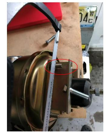
6: Use the MC bracket as a pattern to mark where you have to drill through the firewall and the bracket behind it to fit the 2 additional bolts the new MC requires.
